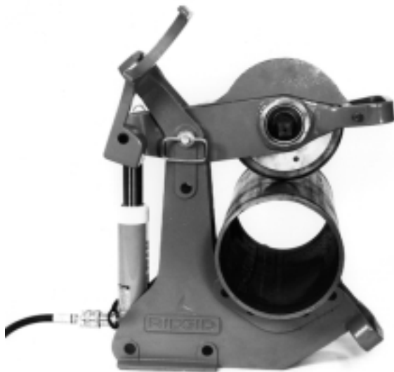
Figure 8 – Positioning Pipe in Cutter
